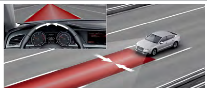
Audi active lane assist (setting 1: early steering intervention)
