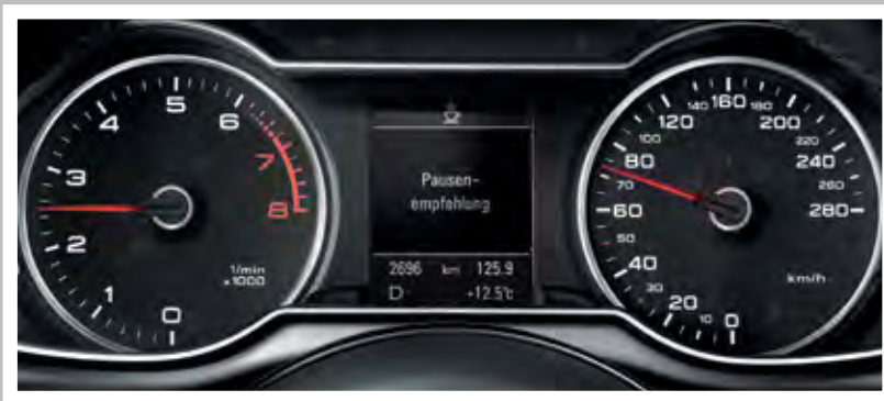
Colour Driver's Information System (DIS) with break recommendation
