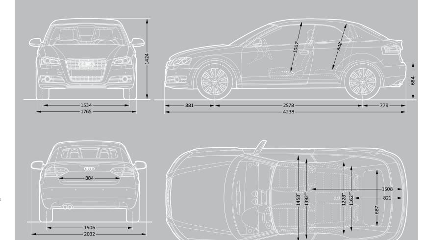
Dimensions were measured with vehicle at unladen weight.
